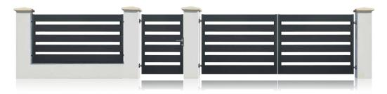
Horizontal infill profiles (P) - 120x20 mm Available options - 40x20; 60x20; 80x20; 100x20 Spacing (S) between profiles - 40 mm U-shape frame - 60x40 mm Spacing can be modified according to the customer's request.
