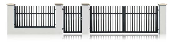
Vertical infill profiles (P) - 20x40 mm Available options - 20x40; 20x60; 20x80 Spacing (S) between profiles - 40 mm U-shape frame - 60x40 mm
