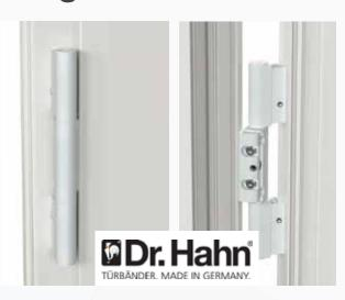
Hinges are strong enough to support doors weighing up to 120 kg weight. Allow door to open up 180°. Hinge diameter 18 mm.
