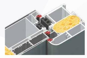
Triple rubber sealing contour provides perfect insulation. D-shape silicone rubber is not ageing or shrinking therefore door insulation does not change during a lifetime.
