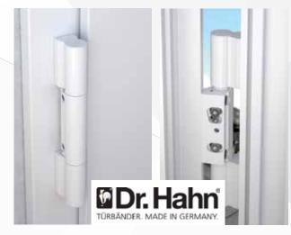
Depending on the design of the profile sections, the 3-piece hinges are able to support doors weighing up to 120 kg. These two series are fastened with the aid of self-drilling screws in the reinforcement of the frame profile with long pins to distribute the forces, acting on the hinge. It also leaves the seal untouched, thus ensuring maintenance of the maximum insulation values. It can be adjusted very conveniently and with little effort in three directions.
